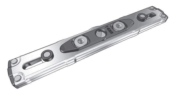
Sterling window lock is a bi-directional stainless steel gearbox for use on aluminium window systems requiring an internal cremone multi point locking system. Patented integrated eurogroove fitting system ensures screwless installation prior to handle fitting.
